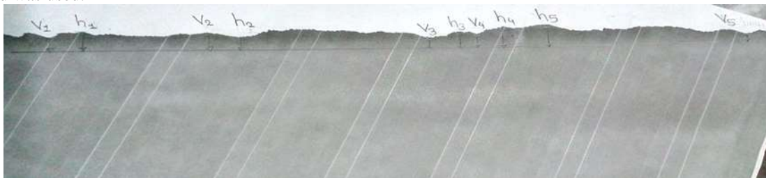
Fig.4. 38 SWG with De-Ionised water (avg roughness)
